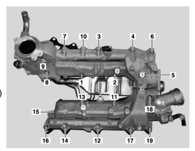
**14 Nm** Fuel rail to cylinder head
